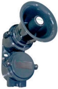
Flameproof Hooter (Sunder) Model : STFH212 Sound Out Put: SPL at 1KHz 110DB Power Supply : 12V, 24V, 48V AC-DC Or 110V, 230V AC
