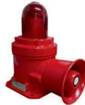
Flameproof Hooter with Flashing Light Model : STFHL100-B Sound Out Put: SPL at 1KHz 110DB Power Supply : 12V, 24V, 48V AC-DC Or 110V, 230V AC
