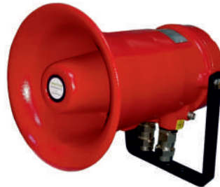
Flameproof PA Loud Speaker (25V) Model : STFH25XT Sound Out Put: SPL at 1KHz 120DB Provided with 100 line Matching Transformer & Taping For 5W / 10W / 15W / 20W / 25W
